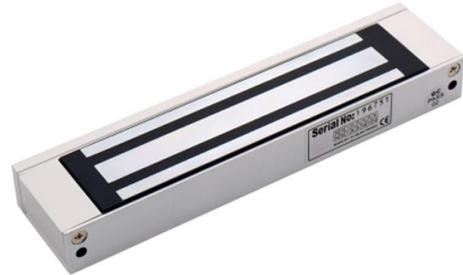
The magnetic lock is designed for wooden door, glass door, and steel door with the opening angle of 90°. The maximum thrust of the lock is 272 kg (599.8 lbs). It can be used for controlling door opening/closing, and the indicator shows the door status. It supports signal output of door lock output status testing.
